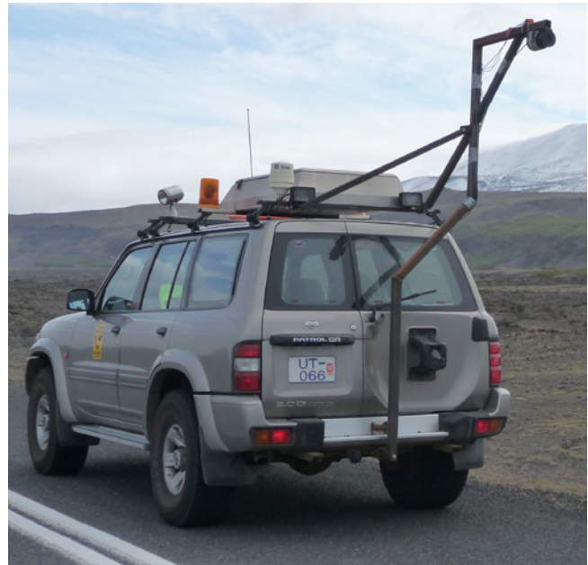
ICERA survey vehicle in Iceland equipped with laser scanner for road speed drainage surveys (photo: Seppo Tuisku)
