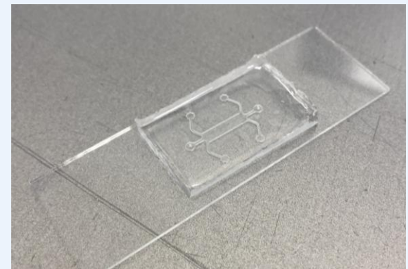
PDMS Microfluidic chip bonded using plasma process
