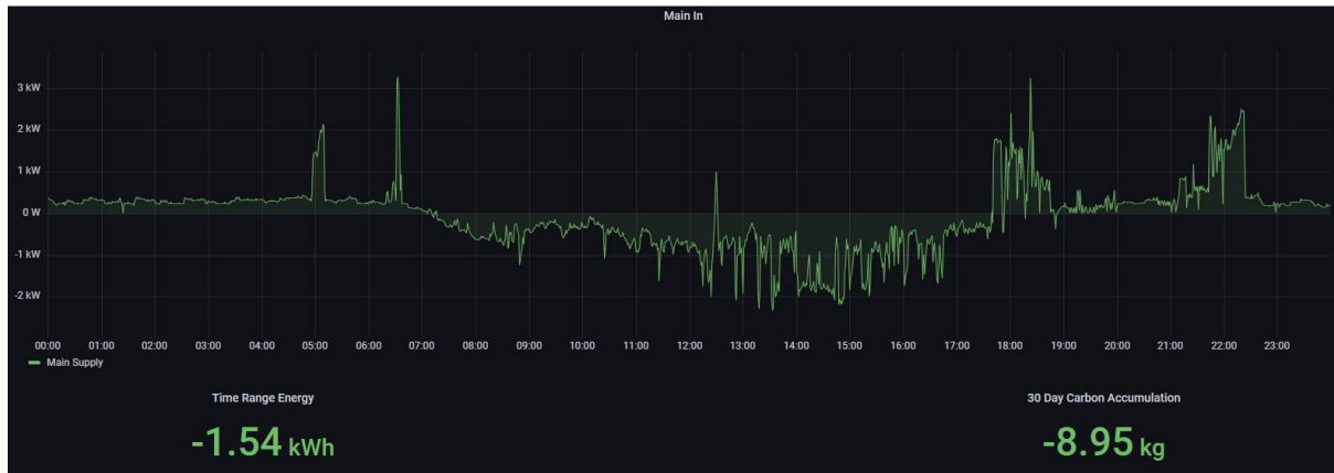
Figure 74. Energy Use and Carbon Accumulation in 24 hrs at Kilworth House (Source DCSix 2024)
