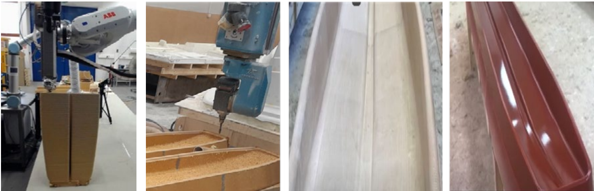
Picture 5. Mould making process: printing, milling, sanding, coating. Photos: Simo Huhtanen.
