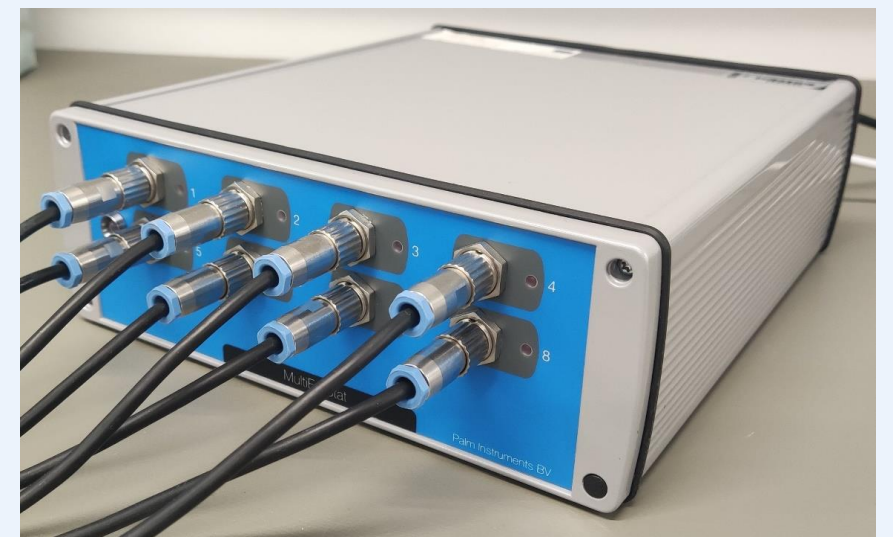
PalmSens 8-channel MultiEmStat2 potentiostat
